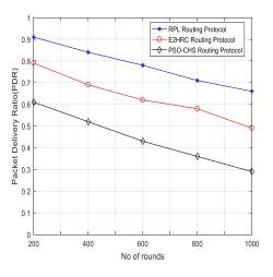
Figure 4.4. PDR comparison of rounds Vs. routing protocols
